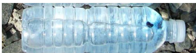
Fig. 1. Coated PET bottle with dye pill (Williams, 2009).
